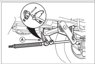
Figure 12. Lift Arm Extension Installation A. Lift Bracket
